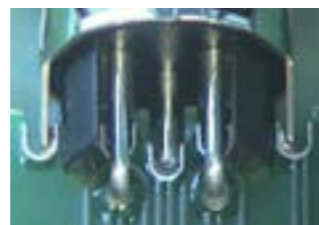
Female solder joints
