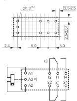
a) Indicated contact position during or after coil energization with reset voltage.
