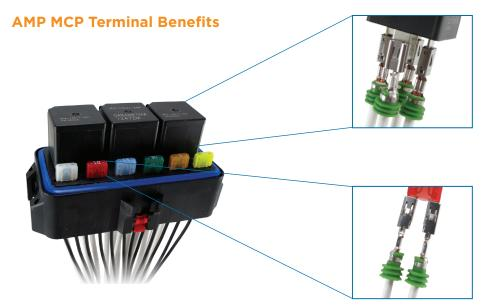
6.3 mm AMP MCP terminal establishes multiple points of contact on both sides of each ISO relay blade terminal, providing stable electrical connection and solid relay retention performance; while 3-gland wire seal provides redundant and robust sealing characteristics to wire and plastic housing.
