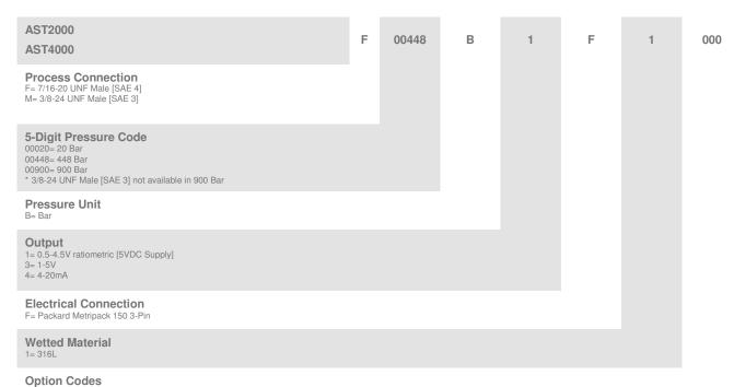
000= Standard. No Options (temp compensation 0 to 55°C) 384= High Accuracy EC79 (temp compensation -20 to 60°C)
