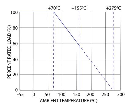
For resistors operated in ambient temperatures above 70°C, power rating must be derated in accordance with this curve.
