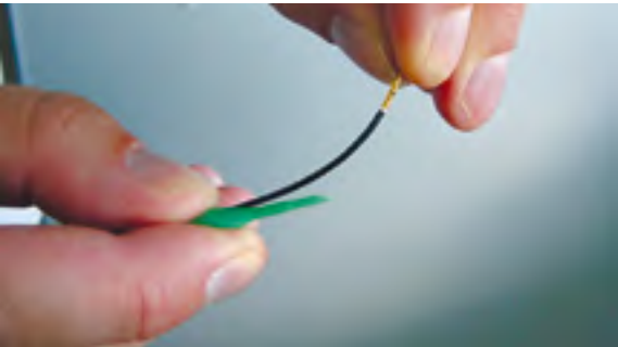
1 After a successful crimp, the contact can now be inserted into the connector. Using the insert/extraction tool provided, slide the wire, using your thumb, so that the wire is enclosed by the tool.
