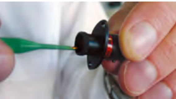
6 Contact being inserted through rear rubber of the connector. Insertion tool should NEVER be rotated, as this will damage the tool and the tines. If the tines get broken the contact may not be retained in the connector.
