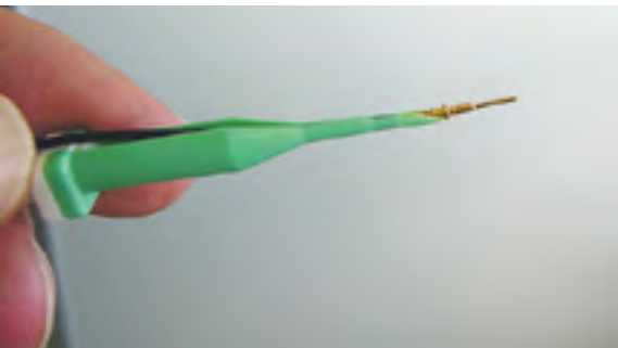
3 After gently pulling the wire through the tool, the contact will now be in position at the end of the tool. The contact should fit securely and the wire should not have any slack.
