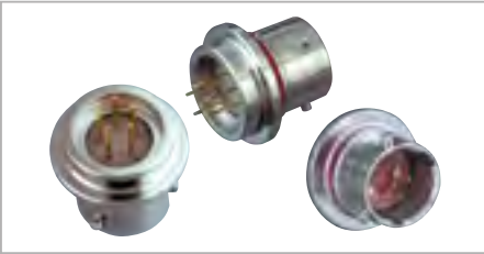
Wildcat UAV Micro HE Hermetic Series Connectors • Filtered Hermetic option also available • Stainless Steel (316) for ease of mounting and corrosion performance • Titanium versions for light weight applications also available • Glass seal can withstand pressure differentials of 1000 psi without loss of electrical performance or fluid leakage Refer to page 33 for additional information on related products.
