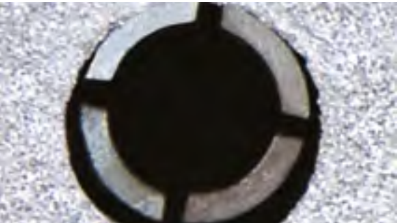
4 This image shows detail of the tines inside the connector. The process of inserting a contact into the connector will slide the contact into position, allowing the shoulder to pass beyond the tines, which will lock into position behind the shoulder. The insertion end of the tool is molded at an angle to ease the contact into position. The extraction end of the tool is molded with a straight end to unlock the tines and allow contact removal.
