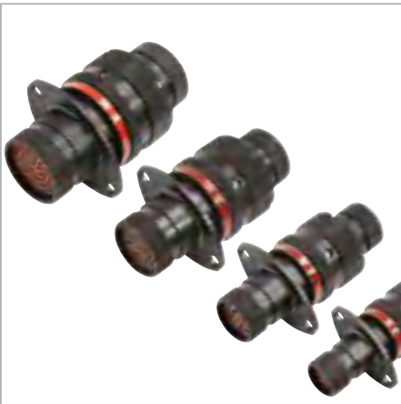
Wildcat UAV Double Density (UAVDD) Series Connectors Next generation connector technology which brings together high density and high performance, inline with using wire size down to AWG 30. The Wildcat UAV Double Density range allows almost double the number of contacts to be packaged in the same shell as compared to the standard Wildcat UAV Series connectors. Refer to page 22 for technical specifications.
