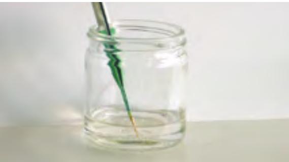
5 This image shows a contact being dipped in IPA to lubricate the insertion process.
