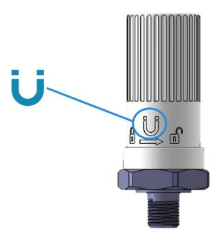
The magnet must be of sufficient strength and proximity to create a magnetic field of 25 mT at the switch location. Two different functions are available depending on the user action:
