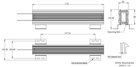
\*This dimension can be adjusted, since threading is available along the length of the resisor.
