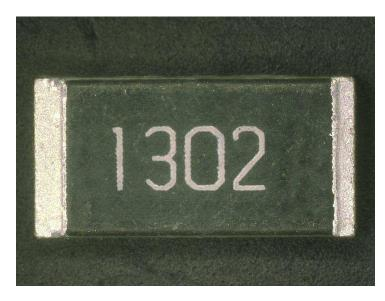
TE Connectivity is pleased to announce that our 3560 high power Thick Film Chip Resistor is now AEC-Q200 Qualified. This sister to our popular 3522 series is suitable for auto placement in volume and for most applications. Supplied as standard on 7 inch Reels of 1000 pieces per reel.
