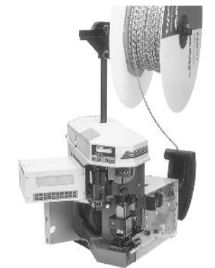
SDE die in PRO-CRIMPER frame. Go to www.tooling.te.com for additional tooling options for SDE dies.
