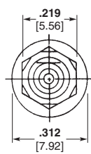
Receptacle, Front Mount Part Number 145-0002-0001
