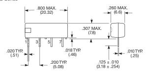
Note: Magnetic shielding may be required between relays when they are placed in very close proximity to one another.
