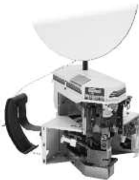
AMP-O-LECTRIC Model "G" Terminating Machine
