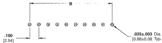
Recommended PC Board Hole Layout (for .062 [1.57] thick PC board)
