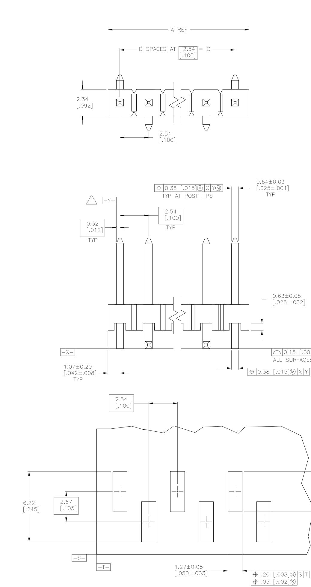
RECOMMENDED PCB LAYOUT FOR USE WITH .008 THICK STENCIL
