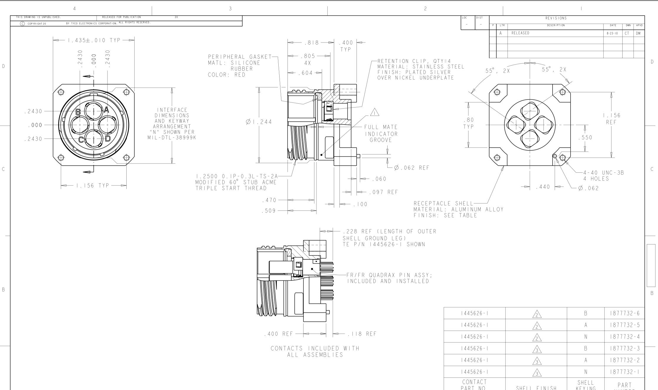
PART IS MARKED WITH Tyco ELECTRONICS CAGE CODE (00779), TE PART NO., Tyco ELECTRONICS LOGO OR TE AND DATE CODE.
