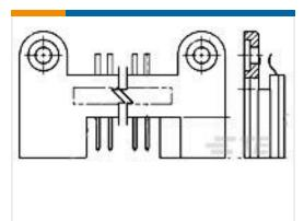
TE Model / Part #583580-1 BOX PIN 50 POS. 100 C/L
