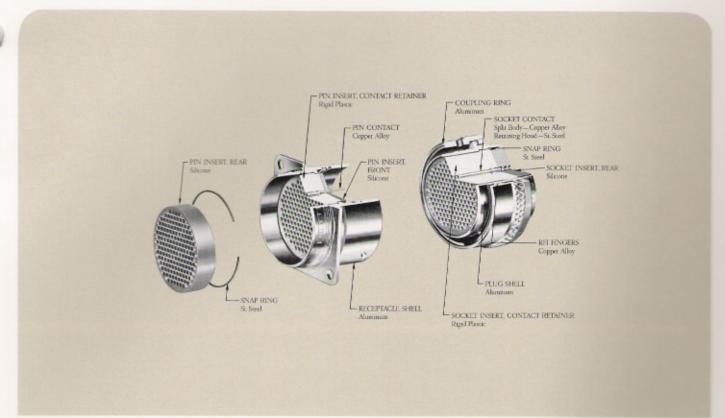
The low contact insertion force inherent in the ICR contact system can reduce assembly time tremendously because in most cases contacts can be inserted into the connector without the use of an insertion tool. Following this simple, single step procedure the contact is positively contained in the connector thereby preventing inadvertent contact release. The integrity of the ICR contact system has been verified by the contact retention system test requirements of MIL-C-81511.
