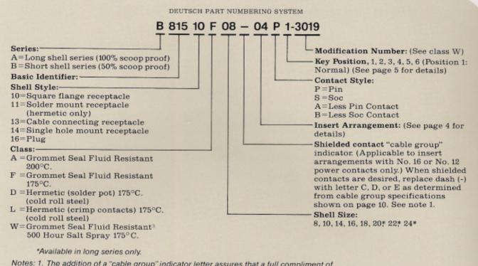
Notes: 1. The addition of a "cable group" indicator letter assures that a full compliment of shielded contacts will be supplied in lieu of the power contacts. If a combination of power and shielded contacts are required within the same arrangement, order a standard connector and, in addition, order the necessary shielded contacts separately. See page 10.
