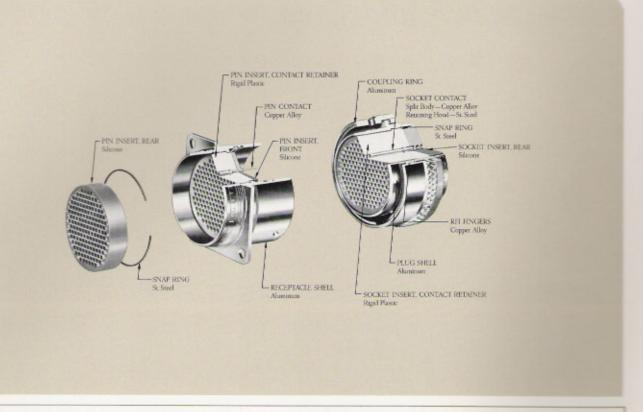
The low contact insertion force inherent in the ICR contact system can reduce assembly time tremendously because in most cases contacts can be inserted into the connector without the use of an insertion tool. Following this simple, single step procedure the contact is positively contained in the connector thereby preventing inadvertent contact release. The integrity of the ICR contact system has been verified by the contact retention system test requirements of MIL-C-81511.
