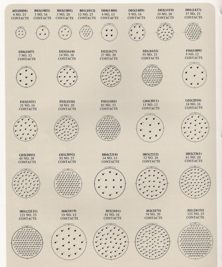
Arrangements are shown looking at pin face (socket is opposite). Cavity identifying numbers are for reference only. Actual marking shall be as required by applicable specifications.
