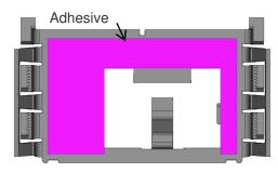
Bracket is specially developed to ensure insertion of sensor in the right way (Poka Yoke ribs), contact of temperature sensor with the windscreen, and maintain of system by adhesive.
