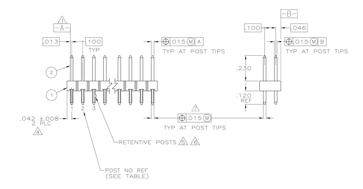
$\overline{-A-}$  shall be the intersection of the post and the housing
