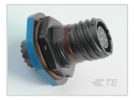
Connector System: Cable-to-Panel Number of Positions: 2 Sealable: Yes Connector & Contact Terminates To: Wire & Cable Contact Current Rating (Max): 13 A
