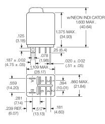
Mounting code 5 Printed circuit terminals
