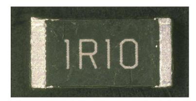
TE Connectivity is pleased to introduce this thick film high power device, sister to our popular 3522 series, suitable for auto placement in volume and for most applications. Supplied as standard on 7 inch Reels of 2000 pieces per reel.
