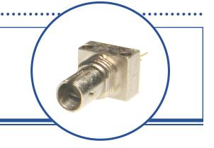
The OPF347 family fiber optic transmitters are high performance devices packaged for data communication links. This transmitter is an 850nm GaAlAs LED and is specifically designed to efficiently launch optical power into fibers ranging in size from 50/125µm up to 200/300µm diameter fiber. Multiple power ranges with upper and lower limits are offered which allows the designer to select a device best suited for the application.
