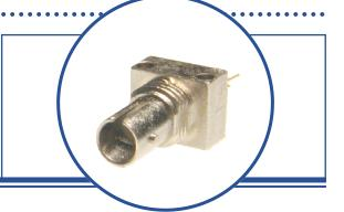
The OPF322 family fiber optic transmitters are high performance devices packaged for data communication links. This transmitter is an 850nm GaAlAs LED and is specifically designed to efficiently launch optical power into fibers ranging in size from 50/125µm up to 200/300µm diameter fiber. Multiple power ranges with upper and lower limits are offered which allows the designer to select a device best suited for the application.
