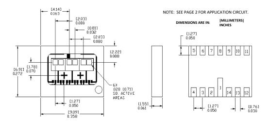
Warning: Front Window is pressure sensitive. Do not apply pressure or high vacuum to window.
