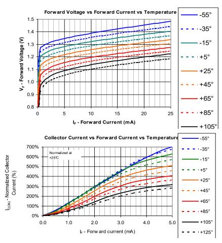
Normalized Collector Current Vs Temperature
