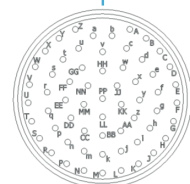
24-61 Service rating 1 61 Contact, Size 24
