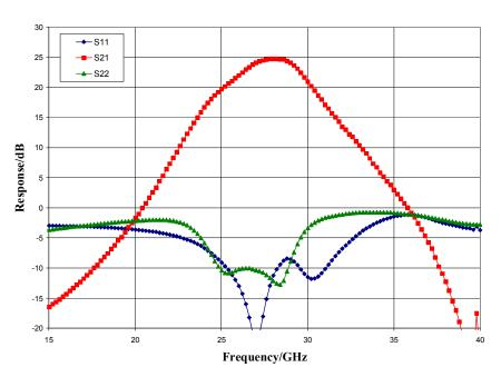
Narrow-band Performance,  $V_{dd} = 28 \text{ V}$ ,  $V_{gg1, 2, 3} = -4 \text{ V}$ ,  $I_{dd} = 350 \text{ mA}$ ,  $T_A = 25 \text{ }^{\circ}\text{C}$
