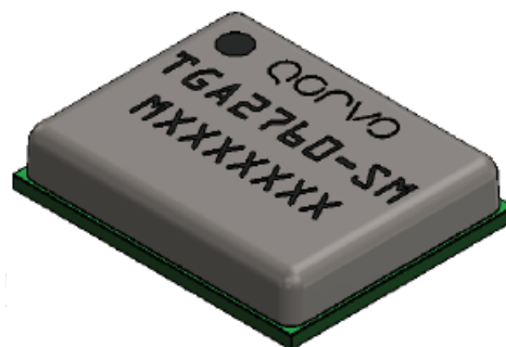
20-Lead 8.0 x 10.0 x 2 mm Package
