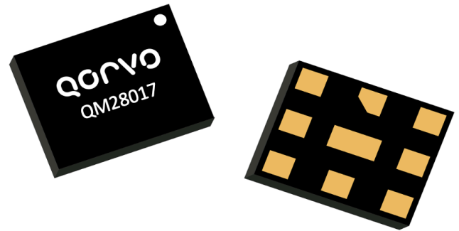
9 Pin 2.0mm x 1.6mm x 0.6mm leadless SMT package
