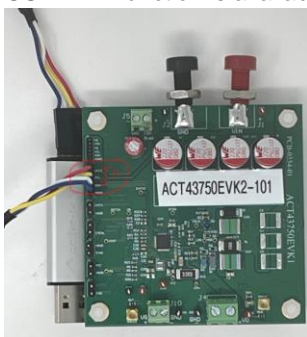
Figure 3. Old dongle connection at J11
