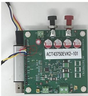
Figure 3. Old dongle connection at J11
