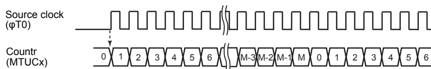
Figure 18-4 Count-up/clear operation when \phi T0 is selected as a source clock
