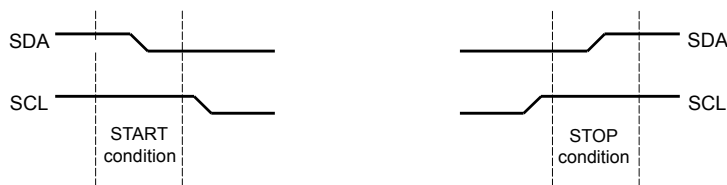
Figure 16-3. START and STOP Conditions
