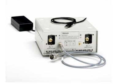
The RTPA2A Real-time Probe Adapter extends the capabilities of Realtime Spectrum Analyzers (RTSA) by offering additional tools to make debugging today's high-performance electrical designs easier. Using the RTPA2A with Tektronix RTSA, design engineers can benefit from industryleading Tektronix active and differential probes to measure signals on SMD pins and other challenging circuit features.
