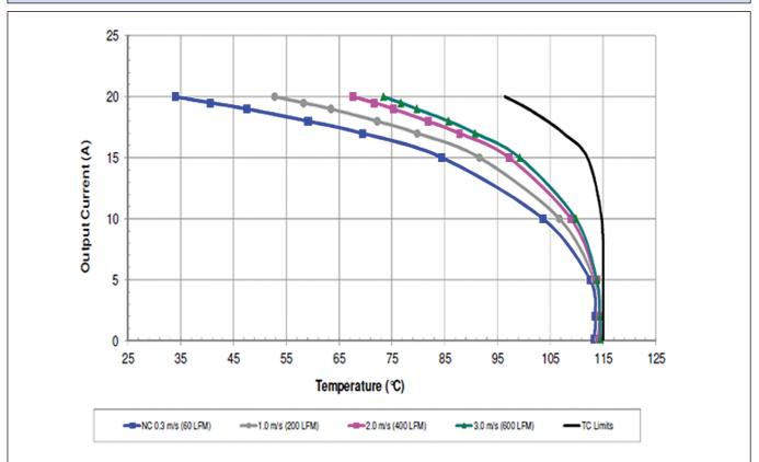
Maxmum output current vs. ambient temperature at nominal input voltage for natural convection (60 LFM) to 400 LFM with airflow from pin 1 to pin 3.
