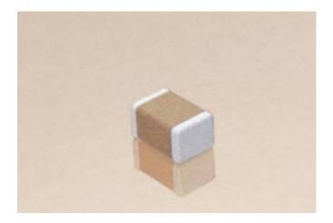
X7R formulations are called "temperature stable" ceramics and fall into EIA Class II materials. X7R is the most popular of these intermediate dielectric constant materials. Its temperature variation of capacitance is within  $\pm 15\%$  from  $-55^{\circ}$ C to  $+125^{\circ}$ C. This capacitance change is non-linear.
