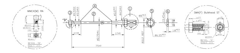
CAB.01044 RG-174 75mm CAB.01046 RG-174 300mm
