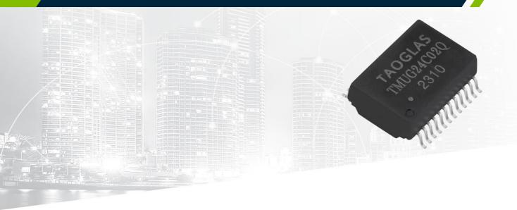
Featuring a compatible footprint with industry LAN transformers, and designed to work in demanding industrial environmental conditions, the Taoglas TMUG24C02Q is a 10G Base-T Single Port of 24pin with Transformer and Common Mode Choke which makes it suitable for PoE+ (720mA) applications in Industrial environments.
