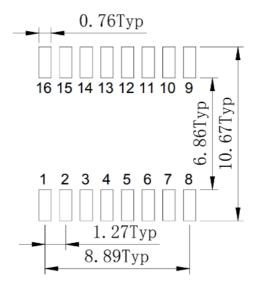
Suggested pad layout Dimensions are in millimeters with the following tolerances: X.XX =  $\pm 0.10$
