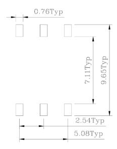
Suggested pad layout Dimensions are in millimeters with the following tolerances:  $X.XX = \pm 0.10$
