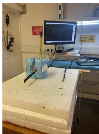
VNA Setup Straight in Free Space
