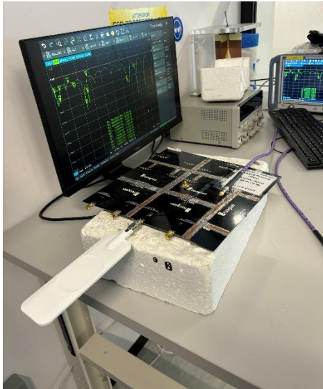
VNA Set up Straight on Edge of 30x30cm Ground Plane
