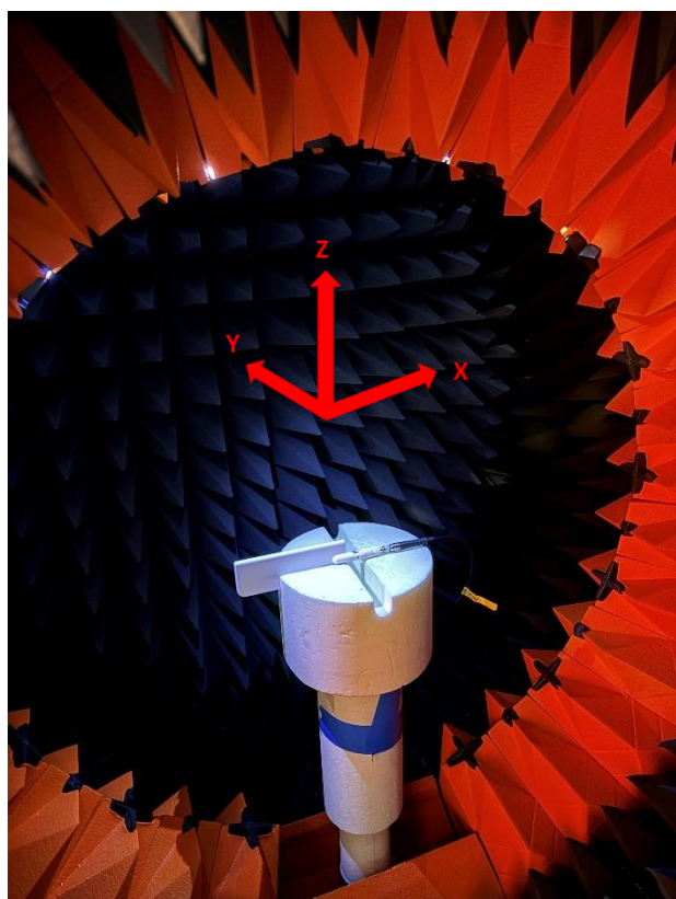
Chamber Set up Straight in Free Space
