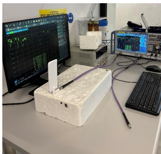
VNA Set up Bent in Free Space
