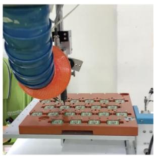
Please note that this process will require a one-time fixture to be made for each PCB design.
