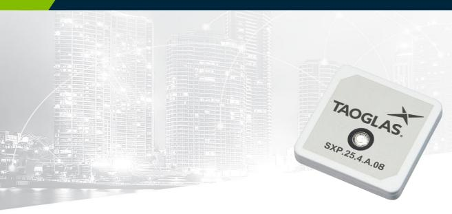
The Taoglas SXP.25.4.A.08 is part of a series of patch antennas designed for use with Satellite Digital Audio Radio Services (SDARS). It features left-hand circular polarization, low in-band axial ratio, and excellent gain characteristics in the 2320 to 2345 MHz band, making it compatible with the most popular satellite radio services available in many new vehicles.
