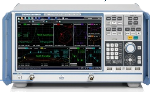
Vector Network Analyzer
