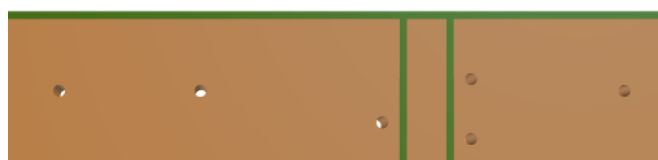
Top View of PCB without Copper Clearance
