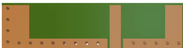
Top View of PCB with Copper Clearance
