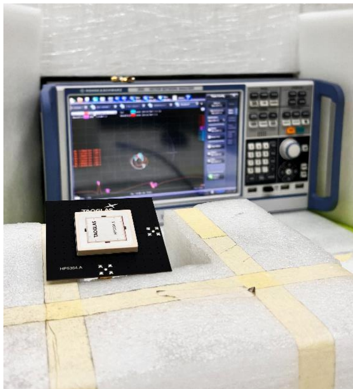
VNA Test Setup on a 70x70mm Ground Plane
