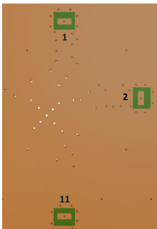
3D Image of Copper Clearances for HP5354.A.
