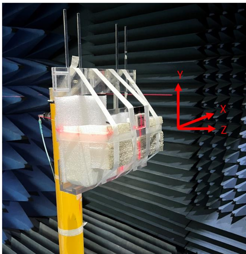
Chamber test setup on 70x70mm ground plane
